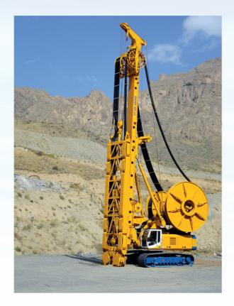
This package includes BG40 drilling mast equipped with rotary means and KDK390 drill bits to drill for high diameter in situ piles as well as excavation means to build deep diaphragm walls complete with grouting accessories and desander.
